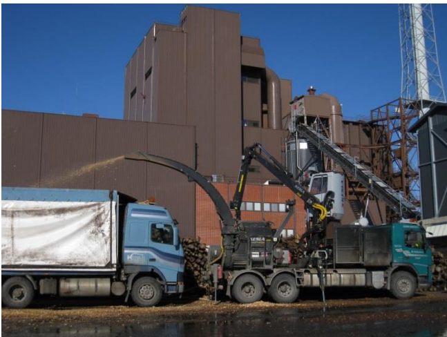
Hybrid chipper by Kesla Oy. Photo: Luke.
