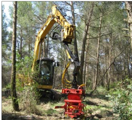
Demonstration of the Naarva Grip EH28 accumulating felling head on 308D CR Caterpillar
