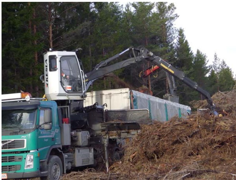
Figure 1 – Chipping pulpwood with the Kesla C 860 H hybrid chipper at the wood terminal in Joensuu (top) and chipping logging residues in Rauma (down).
