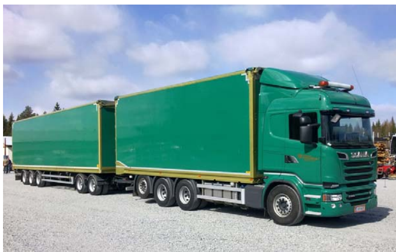
Figure 1. The maximum mass of this chip truck trailer unit is 76 tonnes. Picture: Perttu Anttila.
